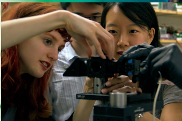
Georgia Squyres, a PhD student in the Molecules, Cells, and Organisms graduate program, adjusts a lens as she builds a microscope.
